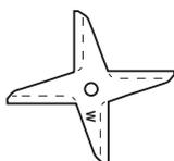
**Wet-Blade Container:** Designed for processing liquids, including juice, frozen mixtures, sauces, soup, purees, batter, and for wet chopping. The wet blades can also process grain and knead dough, but they are not quite as efficient as the dry blades in this application. See instructions for dry container use.
