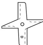
**Dry-Blade Container:** These blades are clearly marked “D” and are designed specifically for processing dry materials such as grain, cereal and coffee, and are also used for kneading bread dough. The dry blades **CANNOT** process liquids efficiently. **If you prepare herbs on a regular basis, you may wish to purchase a separate dry-blade container.**
