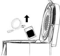
3. Remove the carbon filter cartridge from the main body.
