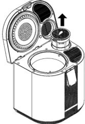
4. Open the carbon filter cartridge by twisting the lid counter-clockwise.
